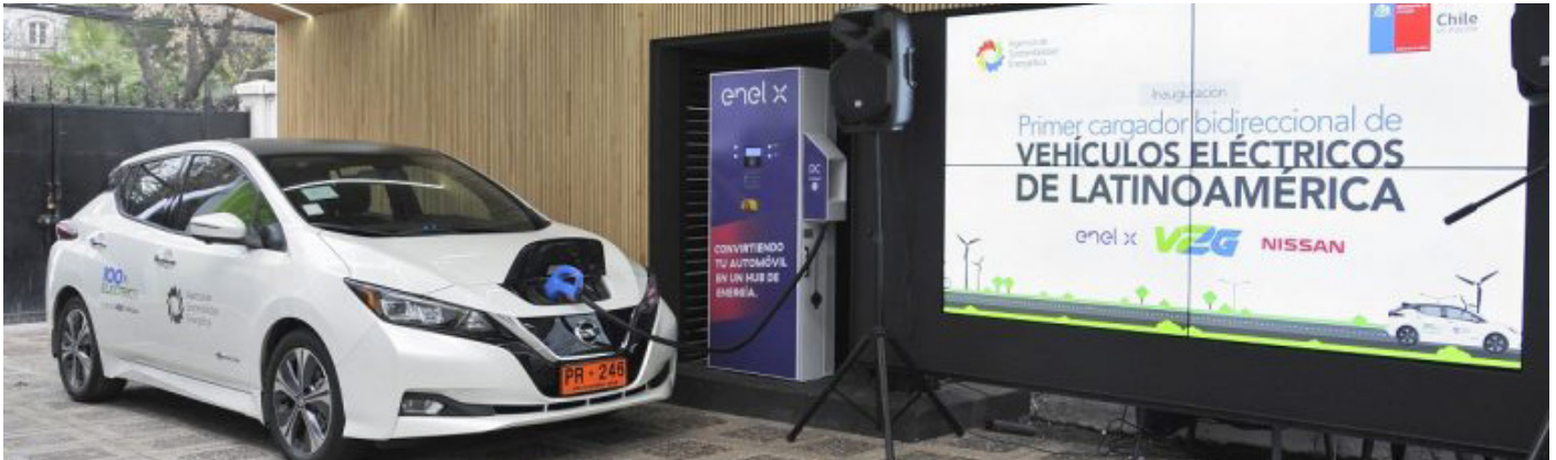
Figure 1. Nissan LEAF charging and discharging electricity at a V2G power station. Source: Nissan Motor Corporation
