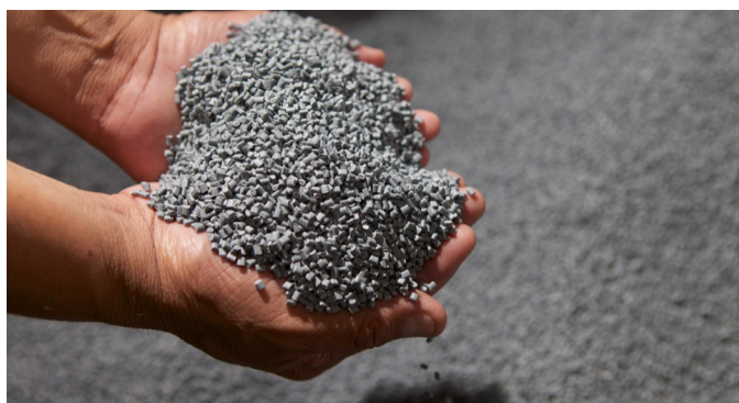
Figure 3. Recycled plastic pellets, colour indicates a degree of contamination. Source: Green Path Recovery
