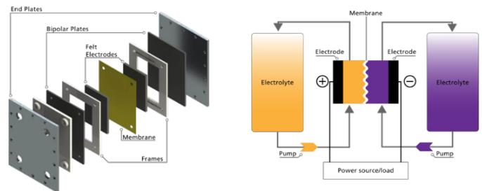
Figure 2. Exploded view and general schematic of a flow battery. Source: FlowCamp
