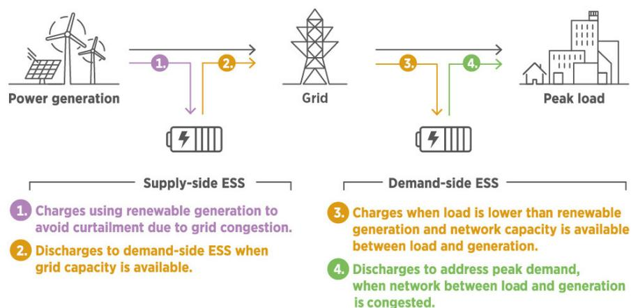
Figure 1: Schematic representation of the virtual power line concept
