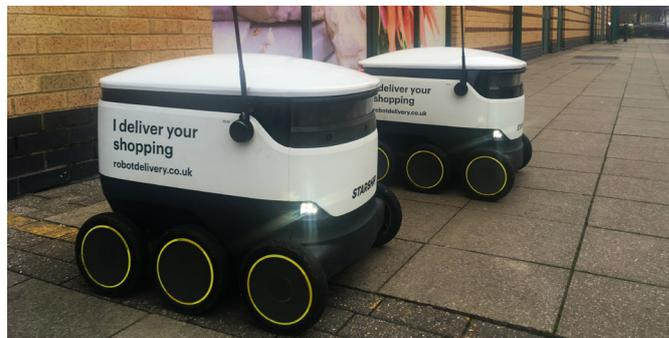
Figure 1. Wheeled delivery robots.
