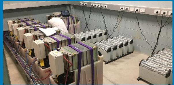
Figure 6. Zinc-bromine flow batteries in a performance testing lab. Source: Simon Hackett
