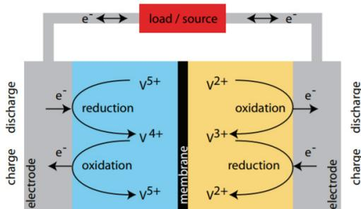
Figure 3. Vanadium redox flow battery charge and discharge process. Source: CDN
