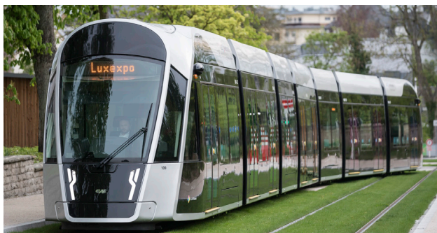
Figure 3. Spain's supercapacitor-powered Greentech Freedrive, Urbos 3 tram. Source: CAF
