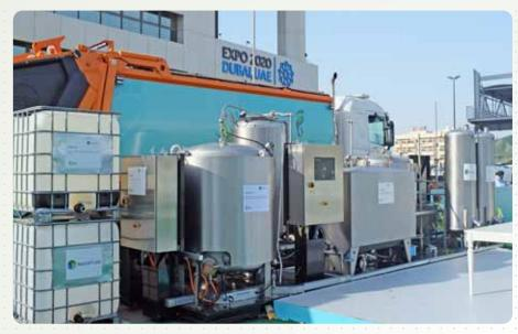
Neutral Fuels' system for producing biodiesel from used cooking oil
