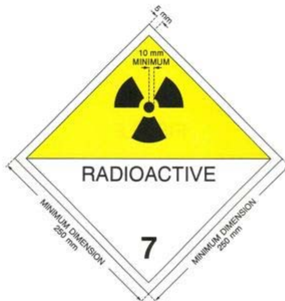
FIGURE 5. Placard. The number “7” shall not be less than 25 mm high. The background colour of the upper half of the placard shall be yellow and of the lower half white, the colour of the trefoil and the printing shall be black.
