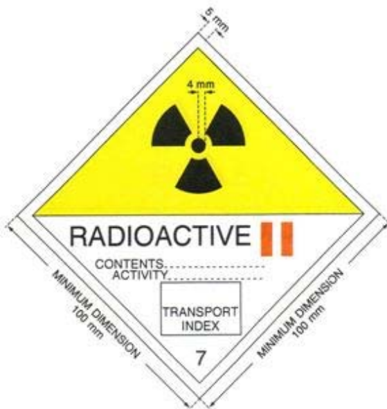
FIGURE 3. Category II-YELLOW label. The background colour of the upper half of the label shall be yellow and the lower half white, the colour of the trefoil and the printing shall be black, and the colour of the category bars shall be red.
