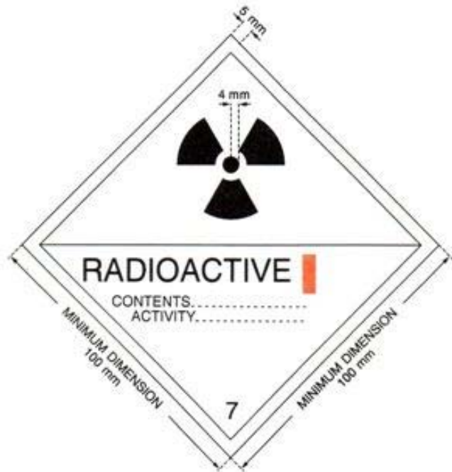
FIGURE 2. Category I-WHITE label. The background colour of the label shall be white, the colour of the trefoil and the printing shall be black, and the colour of the category bar shall be red.
